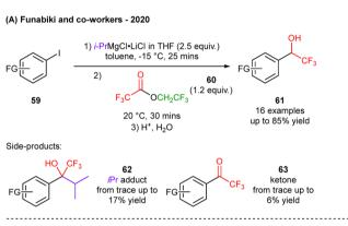
Scheme 10 The application of turbo Grignard reagents with fluoroalkyl esters to form (A)  $\alpha$ -aryl- $\alpha$ -trifluoromethyl alcohols and (B) 1-trifluoromethylated propargyl alcohols.
