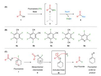
Scheme 1 (A) A nucleophilic substitution from a carboxylic acid mediated by a fluorinated arene based ester with (B) selected examples of compatible fluoroarenes and (C) a general mechanism
