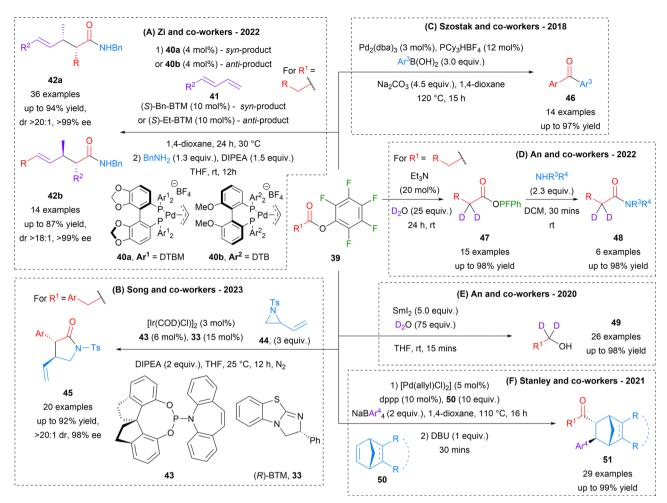
Scheme 8 A selection of transformations from PFPh esters. (A) 1,3-Diene and PFPh ester coupling, (B) γ-lactam synthesis, (C) non-decarbonylative Suzuki-Miyaura cross coupling, (D)  $\alpha$ -deuteration, (E) reductive deuteration and (F) synthesis of bicyclic ketones.
