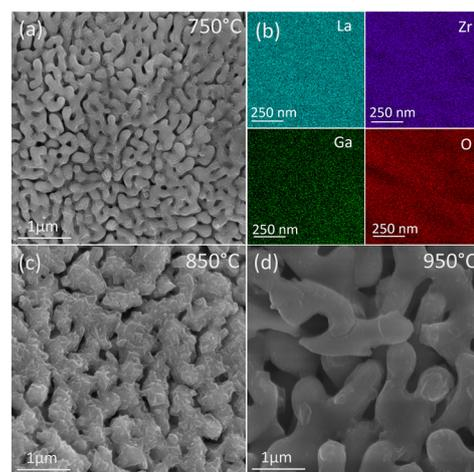
**Fig. 2** FE-SEM images of c-GaLLZO prepared from the precursor mixture-urea composite (F/O = 0.5), calcined at different temperatures for 15 minutes: (a) 750 °C and its corresponding energy-dispersive X-ray (EDX) mapping in (b), (c) 850 °C and (d) 950 °C.
