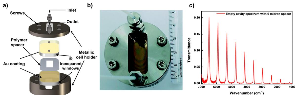
**Fig. 6** Microfluidic cavity for VSC: (a) schematic of a disassembled microfluidic cavity with two parallel gold mirrors forming the FP cavity configuration, (b) picture of an assembled cavity, (c) infrared spectrum of an air-filled cavity [reproduced with permission from ref. 34. Copyright (2022) Royal Society of Chemistry].
