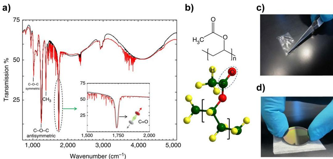
**Fig. 5** Solid-state VSC: (a) infrared spectrum of a PVAc thin film; (b) molecular structure of PVAc, (c) free-standing PVAc thin film, and (d) a solid-state cavity containing spin-coated PVAc sandwiched between two gold mirrors on a germanium substrate [reproduced with permission from ref. 28. Copyright (2015) Springer Nature].
