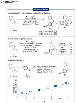
Scheme 3 Key mechanistic findings including (A) reactions with a ruthenacycle, (B) radical scavenger experiments, and (C) on/off experiment.
