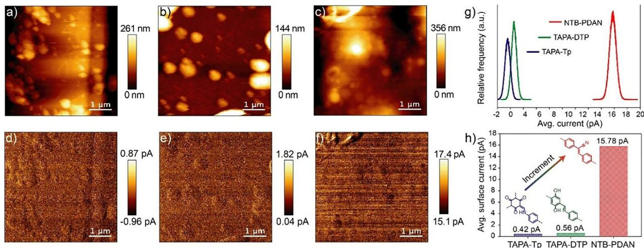
Fig. 2 (a)–(c) Represent the CAFM topographic images of TAPA-Tp, TAPA-DTP, and NTB-PDAN COMs, respectively, while (d)–(f) display their corresponding CAFM current maps at 2 V applied bias on a  $5\text{ }\mu\text{m} \times 5\text{ }\mu\text{m}$  area, and (g) shows the combined current histograms for the COMs, while (h) compares their average surface currents at an applied bias of 2 V.
