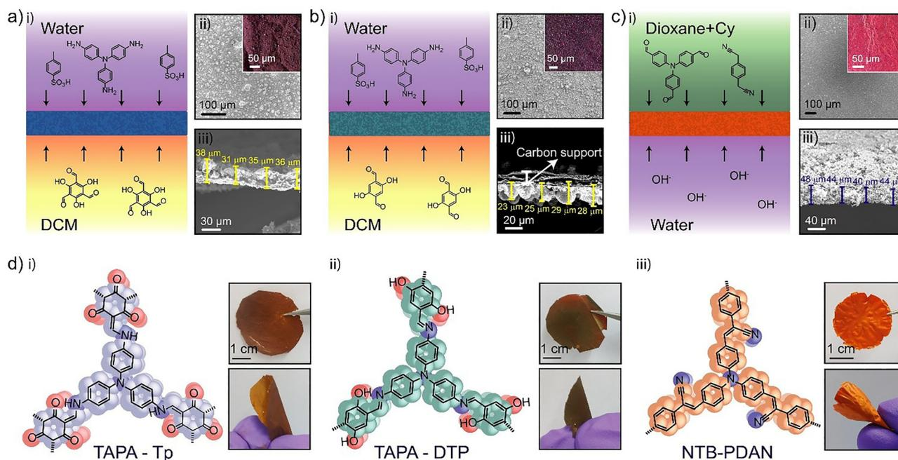
**Fig. 1** Schematic representation of the fabrication (i) along with scanning electron microscopy (SEM) images of the surface (ii) and cross-section (iii) of (a) TAPA-Tp, (b) TAPA-DTP and (c) NTB-PDAN membranes (inset: optical microscopy images); (d) representative model and digital images of (i) TAPA-Tp, (ii) TAPA-DTP and (iii) NTB-PDAN membranes.
