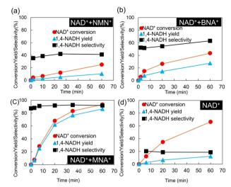
Fig. 4 Production of 1,4-NADH from NAD $^+$  via the hydrogenation of mNAD $^+$ s. Reactions were performed with 8 mmol L $^{-1}$  of (a) NMN $^+$ , (b) BNA $^+$ , or (c) MNA $^+$  and 0.5 mmol L $^{-1}$  NAD $^+$  in 10 mL of 0.1 mol L $^{-1}$  TrisHCl buffer (pH 8.8) at 20 °C. (d) 0.5 mmol L $^{-1}$  NAD $^+$  under the same conditions, without mNAD $^+$ .
