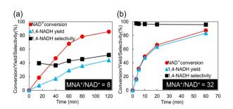
Fig. 5 NAD+ hydrogenation with different MNA+/NAD+ molar ratios. The reaction was carried out in 20 mL of 0.1 mol  $L^{-1}$  Tris–HCl Buffer (pH 8.8) containing NAD+ (0.5 mmol  $L^{-1}$ ) and MNA+ at either (a) 4 mmol  $L^{-1}$  (MNA+/NAD+ = 8) or (b) 16 mmol  $L^{-1}$  (MNA+/NAD+ = 32), using 10 mg of 0.5 wt% Pt/SiO2 catalyst under 1 atm H2 at 20 °C.
