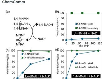
Fig. 3 (a) Production of 1,4-NADH from NAD $^+$  using 1,4-MNMH, 1,4-BNAH, or 1,4-MNAH as hydride donors. Reaction conditions are 8 mmol L $^{-1}$  of (b) 1,4-MNMH, (c) 1,4-BNAH, or (d) 1,4-MNAH and 4 mmol L $^{-1}$  NAD $^+$  in 0.1 mol L $^{-1}$  Tris-HCl buffer (pH 8.8) at 20 °C. The reaction volume was 10 mL.
