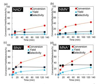
Fig. 2 Hydrogenation of mNAD+s. Reaction conditions: 1.8 mmol L-1 (a) NAD+, (b) NMN+, (c) BNA+, or (d) MNA+ in 20 mL of Tris-HCl buffer (pH 8.8), with 20 mg of 0.5 wt% Pt/SiO $_2$  catalyst, under 1 atm H $_2$ , 20 °C.
