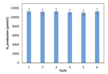
Fig. 3 Reusability test of CeO<sub>2</sub>-MOG for photocatalytic hydrogen production under visible-light irradiation over six consecutive cycles. Reaction conditions: glucose concentration =  $250 \text{ mg L}^{-1}$ ; catalyst dosage =  $2 \text{ g L}^{-1}$ ; solution volume = 80 mL; irradiation time = 4 hours per cycle; light source = four visible-light lamps (8 W each, 400-700 nm).
