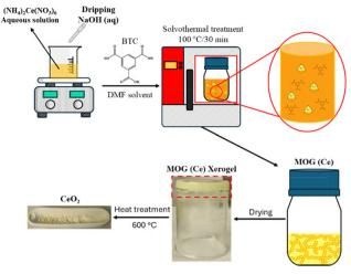
Scheme 1 Scheme of the preparation route of MOG (Ce) and derived CeO2-MOG by heat treatment in air.
