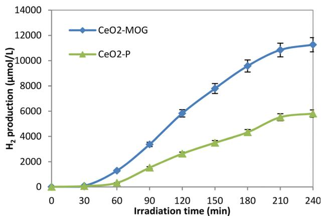
Fig. 2 Hydrogen production over CeO<sub>2</sub>-P (prepared with conventional precipitation synthesis), and CeO<sub>2</sub>-MOG<sub>2</sub> photocatalysts during 4 hours of visible light irradiation. Reaction conditions: catalyst dosage = 2 g L<sup>-1</sup>; initial glucose concentration = 250 mg L<sup>-1</sup>; solution volume = 80 mL; light source = four visible light lamps (8 W each, 400–700 nm).
