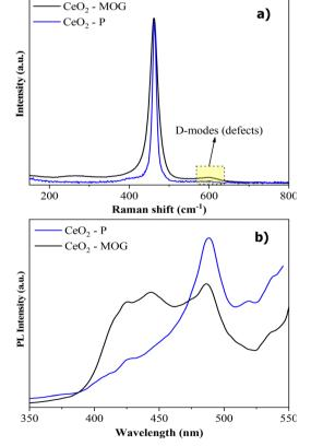
Fig. 1 (a) Raman spectra of CeO<sub>2</sub>-P and CeO<sub>2</sub>-MOG photocatalysts. (b) Photoluminescence spectra of CeO<sub>2</sub>-P and CeO<sub>2</sub>-MOG samples.
