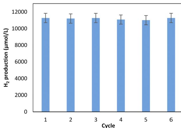
Fig. 3 Reusability test of CeO<sub>2</sub>-MOG for photocatalytic hydrogen production under visible-light irradiation over six consecutive cycles. Reaction conditions: glucose concentration = 250 mg L<sup>-1</sup>; catalyst dosage = 2 g L<sup>-1</sup>; solution volume = 80 mL; irradiation time = 4 hours per cycle; light source = four visible-light lamps (8 W each, 400–700 nm).
