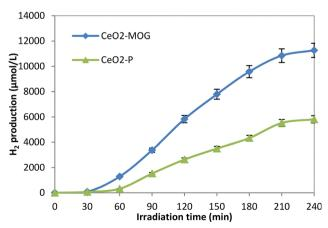
Fig. 2 Hydrogen production over CeO<sub>2</sub>-P (prepared with conventional precipitation synthesis), and CeO<sub>2</sub>-MOG<sub>2</sub> photocatalysts during 4 hours of visible light irradiation. Reaction conditions: catalyst dosage =  $2 \text{ g L}^{-1}$ ; initial glucose concentration =  $250 \text{ mg L}^{-1}$ ; solution volume = 80 mL; light source = four visible light lamps (8 W each, 400-700 nm).
