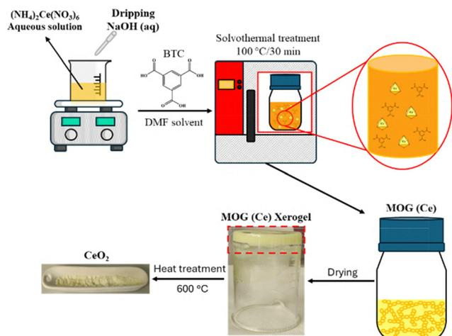
**Scheme 1** Scheme of the preparation route of MOG (Ce) and derived CeO<sub>2</sub>-MOG by heat treatment in air.
