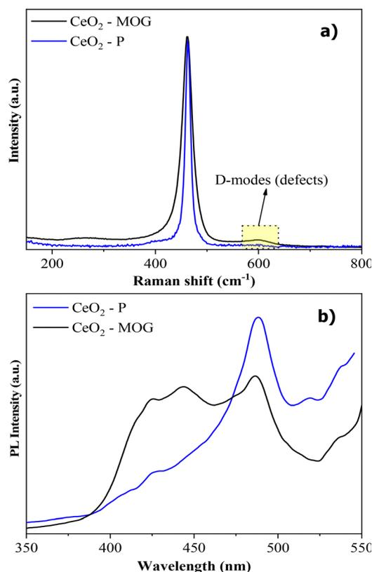
**Fig. 1** (a) Raman spectra of CeO<sub>2</sub>-P and CeO<sub>2</sub>-MOG photocatalysts. (b) Photoluminescence spectra of CeO<sub>2</sub>-P and CeO<sub>2</sub>-MOG samples.
