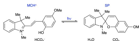
**Scheme 1** Photoisomerisation of the protonated merocyanine (MCH<sup>+</sup>) to spiropyran (SP) and its application to seawater CO<sub>2</sub> capture and release.
