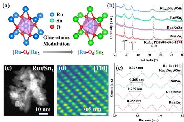
Fig. 1 (a) Schematic illustration of composition design based on cluster-plus-glue-atom model. (b) XRD patterns of Ru–Sn oxides. (c) low and (d) high-magnification HAADF-STEM images of Ru#Sn<sub>2</sub>. (e) Scans of the (101) lattice distance of Ru–Sn oxides.
