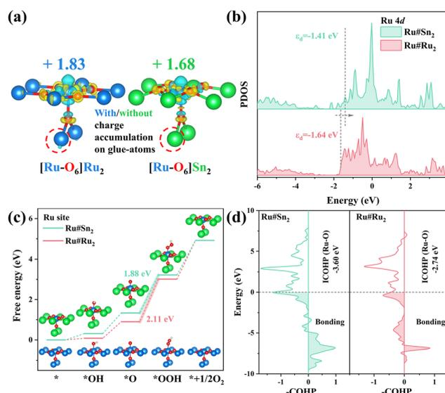
Fig. 4 (a) Differential charge density and Bader charge calculation of Ru#Ru<sub>2</sub> and Ru#Sn<sub>2</sub>. (b) The PDOS of Ru 4d for Ru#Ru<sub>2</sub> and Ru#Sn<sub>2</sub>. (c) Gibbs free energy diagrams on Ru site at  $U = 0$  V for Ru#Ru<sub>2</sub> and Ru#Sn<sub>2</sub>. (d) COHP of Ru#Sn<sub>2</sub> and Ru#Ru<sub>2</sub>.
