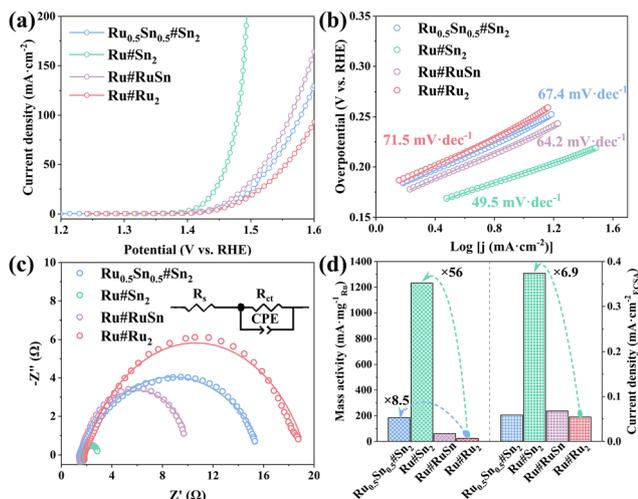
Fig. 3 Electrochemical OER performance evaluation for Ru–Sn oxides in 0.5 M H<sub>2</sub>SO<sub>4</sub>. (a) LSV polarization curves, (b) Tafel plot. (c) Nyquist plots of EIS and fitting result with equivalent circuit. (d) Ru mass activities and ECSA normalized activities of Ru–Sn oxides at potentials of 1.50 V (vs. RHE).
