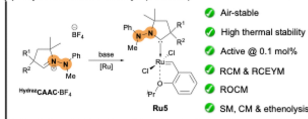
Fig. 1 State of the art of CAAC–Ru complexes for olefin metathesis (a) and the development of a new CAAC–Ru complex featuring an N -hydrazine unit (b, this work).
