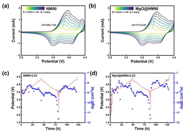
Fig. 3 Cyclic voltammogram of (a) NM90 and (b) MgO@NM90 at rates from 0.1 to 0.7 mV s<sup>-1</sup>. Li<sup>+</sup> diffusion coefficient calculated via GITT of (c) NM90 and (d) MgO@NM90.
