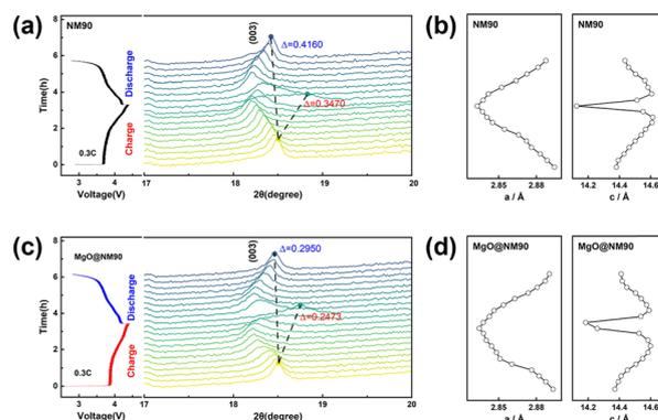
Fig. 4 *In situ* XRD (003) patterns and corresponding voltage curves during the initial cycle at 0.3C for (a) NM90 and (c) MgO@NM90. Lattice parameter evolution derived from the *in situ* XRD patterns for (b) NM90 and (d) MgO@NM90.
