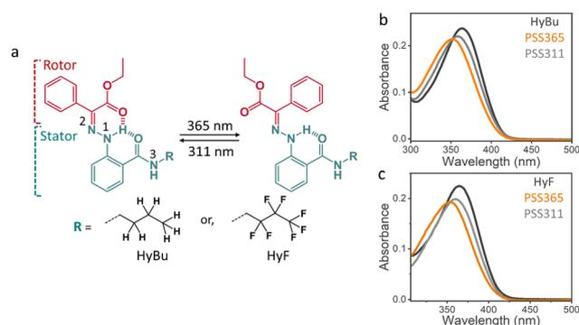
**Fig. 1** (a) Molecular structures of the *Z*-isomers of **HyF** and **HyBu**. Light induced *Z/E* isomerisation. N atoms are numbered to aid discussion. Changes in absorbance spectra of (b) **HyBu** and (c) **HyF** on forward (365 nm) and backward (311 nm) photoirradiation in ethanol (15  $\mu$ M).
