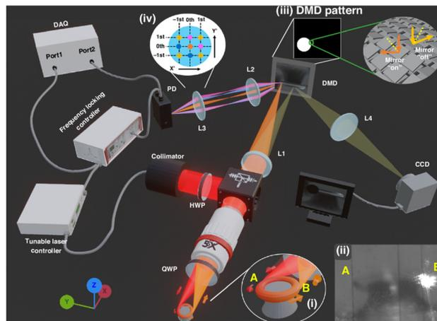
Fig. 9 Free-space coupling system for microtoroid resonance tracking. A  $5\times$  objective lens is used to collimate the incident light and the scattered light at  $180^\circ$  from the incident direction. The collimated light is directed to a digital micromirror device (DMD) and then to a photodetector (PD) for resonance wavelength observation. Reproduced with permission from ref. 80. Copyright © 2024, The Author(s).
