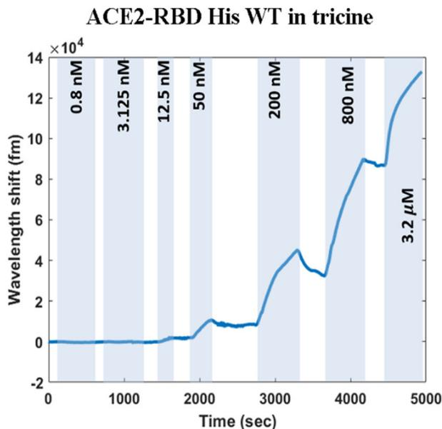
Fig. 4 Wavelength shift of the FLOWER system showing binding of Spike-RBD-His wildtype (WT) to hACE2 in tricine buffer. Blue-shaded regions indicate exposure to increasing concentrations of Spike-RBD, while unshaded regions correspond to running buffer rinses. Reproduced from ref. 21. With permission from the American Chemical Society, copyright 2024.
