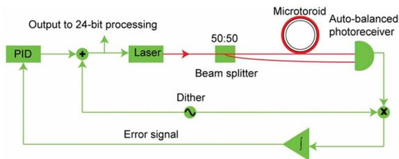
**Fig. 2** Block diagram of the FLOWER system. A frequency-modulated laser generates a signal that, when mixed with a dither signal, produces an anti-symmetric error signal. The error signal is processed by a proportional-integral-derivative (PID) controller, which dynamically adjusts the laser frequency to maintain resonance stability. Reproduced from ref. 20 with permission from the American Chemical Society, copyright 2015.
