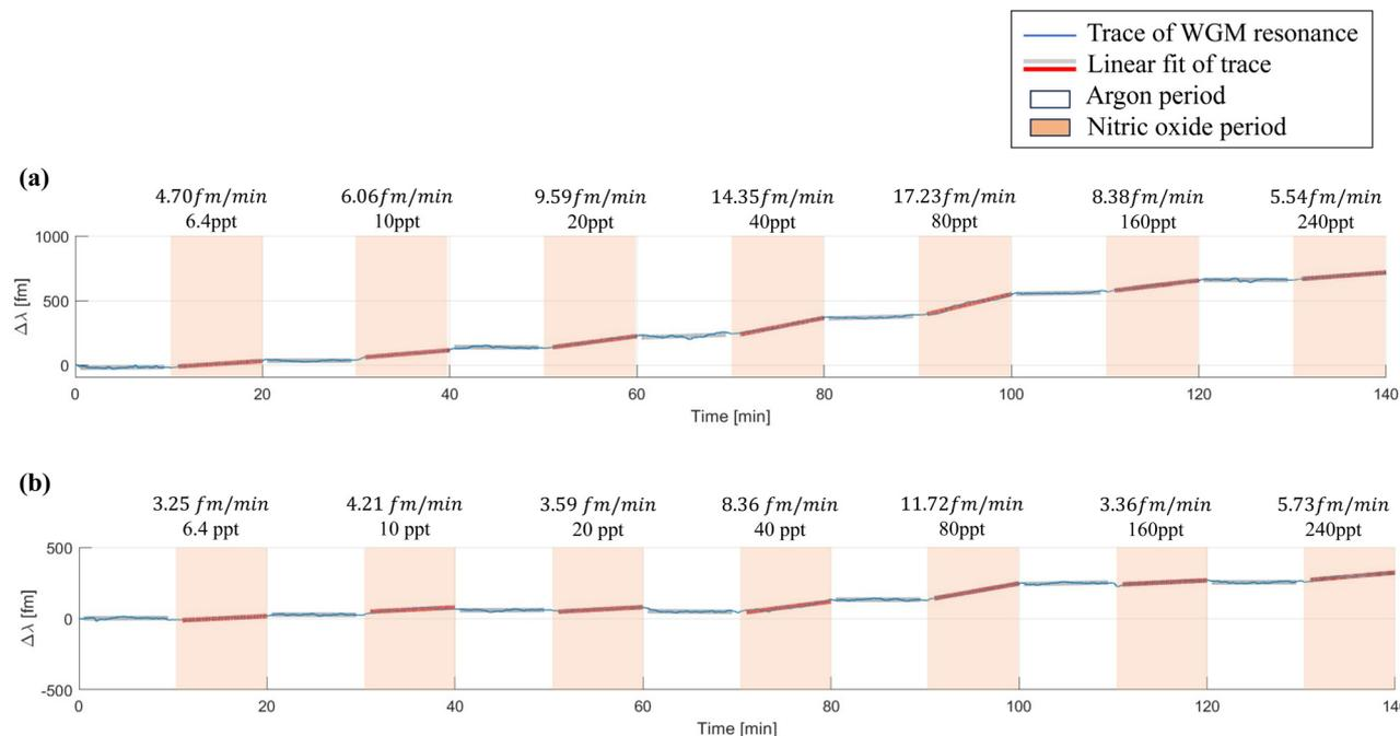
**Fig. 6** Detection of nitric oxide using FLOWER sensors with FcMA/MMA copolymers of varying compositions. (a) Higher FcMA content; (b) higher MMA content. Shaded regions indicate nitric oxide exposure; unshaded regions denote argon. Reproduced from ref. 26 with permission from the American Chemical Society, copyright 2024.
