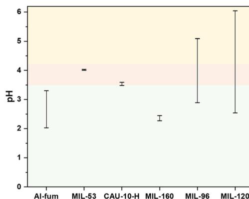
**Fig. 5** pH ranges of all syntheses (first point at reaction start and second after 24 hours). The green zone represents the predominance of  $\text{Al}^{3+}$  species, the red zone is an in-between where plural ionic species exist, and the yellow one is the limit from which aluminium hydroxide starts forming.
