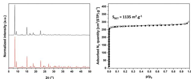
**Fig. 4** PXRD pattern (left) and  $\text{N}_2$  adsorption/desorption isotherm at 77 K (right) of the pilot batch spray-dried MIL-160 sample.
