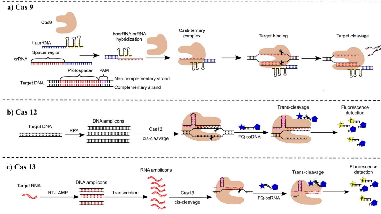
Fig. 2 Detection mechanisms of different Cas effectors. (a) Schematic illustration of Cas 9-based *cis*-cleavage for dsDNA target. (b) Schematic of Cas12-induced *cis*-cleavage and *trans*-cleavage (non-target cleavage) mechanism for dsDNA target detection. (c) Schematic of Cas13-assisted *cis*-cleavage and *trans*-cleavage (non-target cleavage) for ssRNA target detection.<sup>17</sup>
