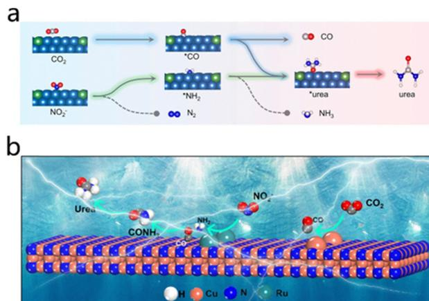
Fig. 3 (a) Urea synthesis from  $\text{CO}_2\text{RR}$  and  $\text{NO}_2\text{RR}$  on Te–Pd NCs. Reproduced with permission from ref. 32. Copyright 2020, Nano Letters. (b) Schematic of the ECNU process on  $\text{Ru}_1\text{@Cu}_3\text{N}$ . Reproduced with permission from ref. 33. Copyright 2024, Chemical Engineering Journal.
