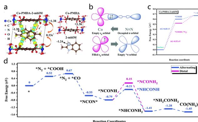
**Fig. 9** (a) The charge density difference of Co-PMDA-2-mbIM and the corresponding results of Bader charge analysis. (b) A simplified schematic diagram of  $\text{N}_2$  bonding to a Co center. (c) Free energy diagrams for  $\text{CO}_2$  reduction with and without  $\text{N}_2$  adsorption on Co-PMDA-2-mbIM. (d) The possible urea electro-synthesis mechanism. Reproduced with permission from ref. 55. Copyright 2022, Energy & Environmental Science.
