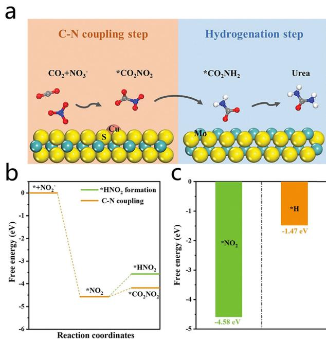
**Fig. 8** (a) Schematic diagram of the tandem catalytic mechanism on  $\text{Cu}_1\text{-MoS}_2$ . Reproduced with permission from ref. 50. Copyright 2024, Advanced Energy Materials. (b) Free energy diagrams of C–N coupling and  $^*\text{HNO}_2$  formation on  $\text{W}_1\text{-S}_3$ . (c) Adsorption free energies for  $\text{NO}_2^-$  and H adsorption on  $\text{W}_1\text{-S}_3$ . Reproduced with permission from ref. 52. Copyright 2025, Journal of Colloid and Interface Science.
