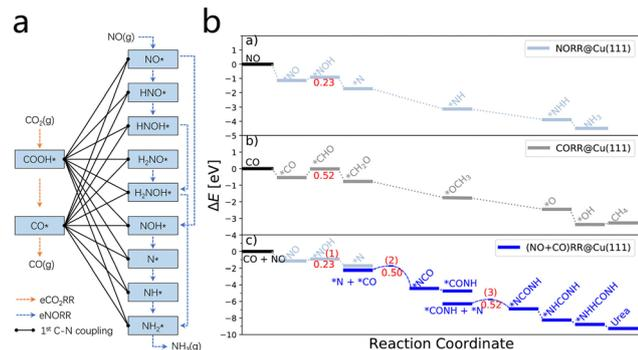
Fig. 4 (a) Schematic illustration of eCO<sub>2</sub>RR, eNORR, and the first C–N coupling reactions. Reproduced with permission from ref. 34. Copyright 2024, ACS Catalysis. (b) Three reaction pathways on the Cu(111) surface energy diagram. Reproduced with permission from ref. 36. Copyright 2023, ACS Catalysis.
