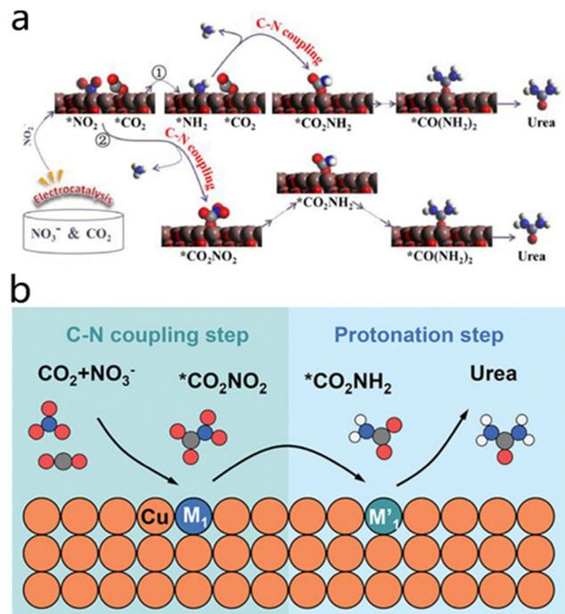
Fig. 2 (a) Two possible pathways for urea synthesis involving  $\text{CO}_2$  and  $\text{NO}_3^-$ . Reproduced with permission from ref. 30. Copyright 2024, Chinese Chemical Letters. (b) Schematic of the tandem catalytic mechanism on Cu DAA. Reproduced with permission from ref. 31. Copyright 2024, Advanced Materials.
