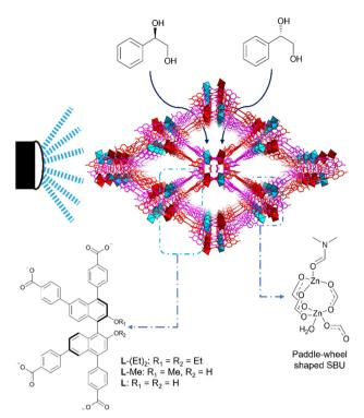
Fig. 1 Schematic illustration of isostructural CMOFs built from Zn<sub>2</sub> paddle-wheel SBUs and BINOL-based tetrabenzoate ligands and their application in luminescence sensing of PE enantiomers.
