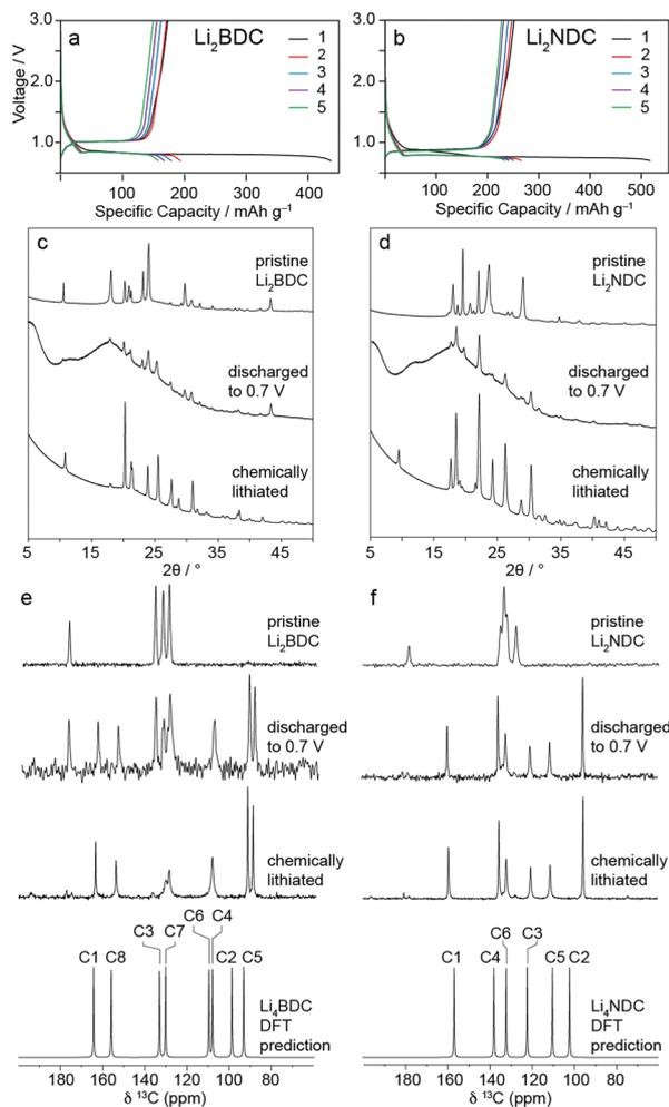
**Fig. 1** (a) and (b) Charge–discharge profiles of  $\text{Li}_2\text{DC}$  electrodes cycled at C/20. (c) and (d) PXRD patterns of pristine, electrochemically discharged, and chemically lithiated  $\text{Li}_2\text{DC}$ s. (e) and (f)  $^{13}\text{C}$  CPMAS NMR spectra of pristine, electrochemically discharged, and chemically lithiated  $\text{Li}_2\text{DC}$ s, and DFT-predicted spectra for SCXRD  $\text{Li}_4\text{DC}$  structures.
