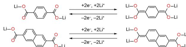
**Scheme 1** Reaction scheme for the reversible reductive lithiation of Li<sub>2</sub>BDC and Li<sub>2</sub>NDC.
