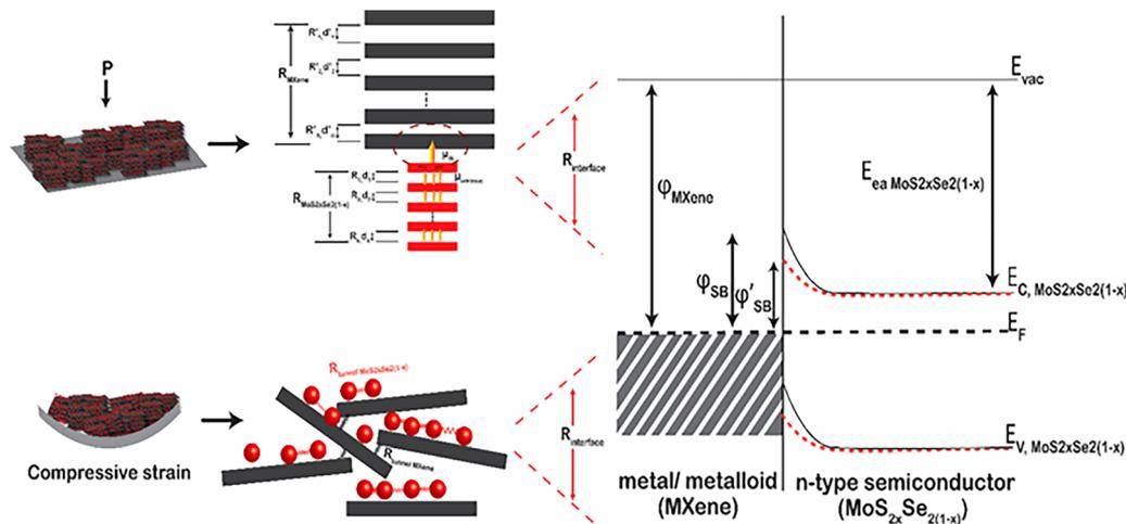
Fig. 5 Percolation network for the pressure and strain sensing mechanism.<sup>113</sup>
