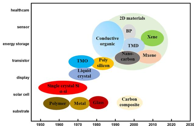
Fig. 1 Timeline of different materials in the development of flexible sensors.
