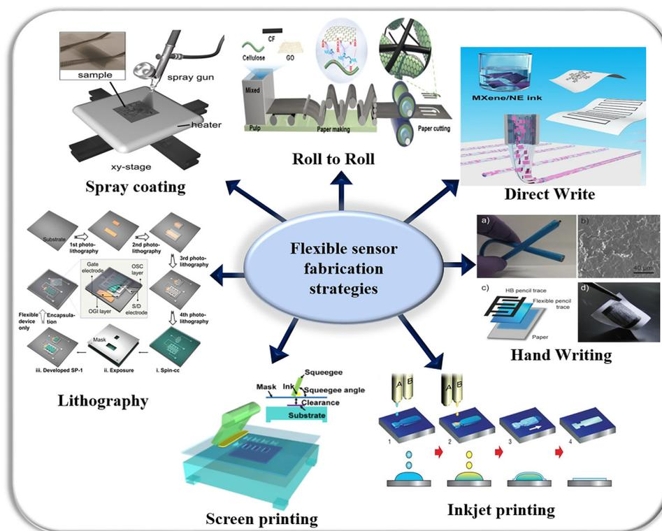
Fig. 4 Process for the fabrication of 2D materials for flexible and wearable electronics applications: roll to roll,<sup>70</sup> direct writing,<sup>55</sup> hand writing,<sup>71</sup> inkjet writing,<sup>73</sup> screen printing,<sup>69</sup> lithography,<sup>72</sup> and spray coating.<sup>49</sup>
