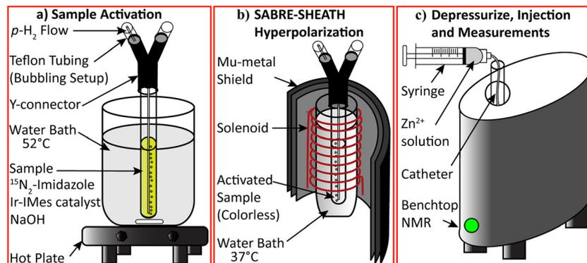
Fig. 2 Schematic diagram depicting the process of  $\text{Zn}^{2+}$  sensing using hyperpolarized  $^{15}\text{N}_2$ -imidazole. (a) The sample was activated by bubbling  $p\text{-H}_2$  while it was in a heated water bath. (b) The activated sample was hyperpolarized in the mu-metal shield by bubbling  $p\text{-H}_2$  at an optimized polarization transfer field. (c) The hyperpolarized solution was transferred to the benchtop NMR, depressurized, and the target ( $\text{Zn}^{2+}$ ) was injected.
