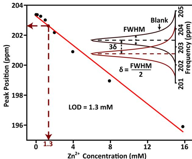
Fig. 5 Calibration curve for  $\text{Zn}^{2+}$  sensing with hyperpolarized  $^{15}\text{N}_2$ -imidazole. A linear correlation between the  $^{15}\text{N}_2$ -imidazole peak shift and  $\text{Zn}^{2+}$  concentration is identified ( $R^2 = 0.984$ ). LOD estimation is depicted, with the blank measurement (black) separated from the subsequent measurement (brown) by  $3\delta$ , yielding a LOD value of 1.3 mM.
