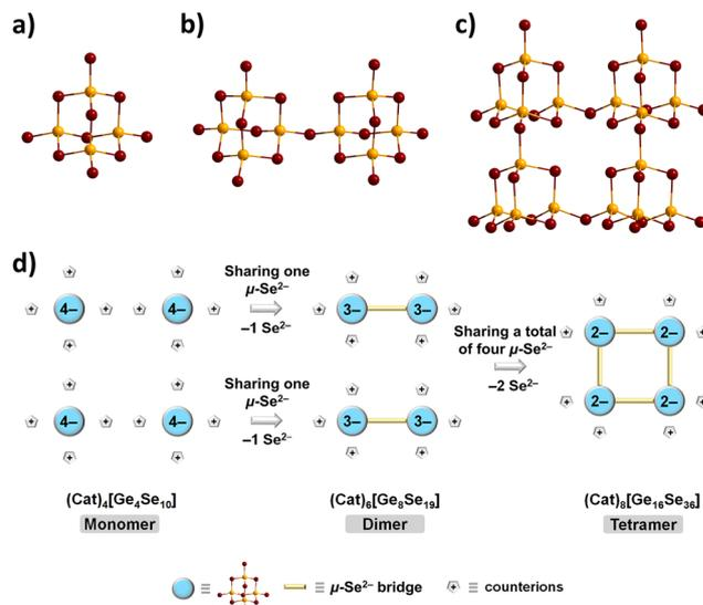
Fig. 3 Structure of the anions in (a)  $(C_2C_1Im)_4[Ge_4Se_{10}]$ , (b)  $(C_2C_1Im)_6-[Ge_8Se_{19}]$  and (c)  $(C_2C_1Im)_8[Ge_{16}Se_{36}]$ . (d) Schematic representation of the strategy for reducing the average charge of supertetrahedral chalcogenido cluster anions through the formation of discrete cluster oligomers. Panel (d) adopted with permission from ACS. Colour code: Ge = light orange, Se = dark red.
