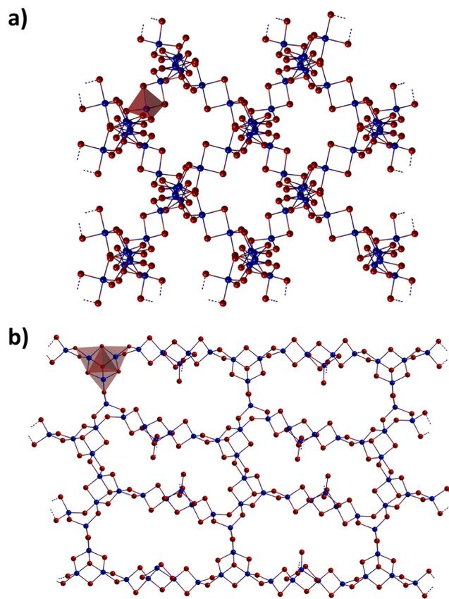
Fig. 5 (a) 3D open-framework of the anion in (C<sub>4</sub>C<sub>1</sub>Im)<sub>4</sub>[Sn<sub>9</sub>Se<sub>20</sub>], and (b) 2D nanotube structure of the anion in (C<sub>5</sub>C<sub>1</sub>Im)<sub>8</sub>[Sn<sub>17</sub>Se<sub>38</sub>]. Colour code: Sn = dark blue, Se = dark red.
