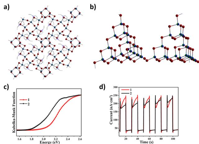
**Fig. 9** (a) Crystal structure of the 3D-open-framework compound  $(C_2H_5Py)[GaSn_2Se_6] \cdot 1/4H_2O$ . (b) Connection of pseudo-T4 supertetrahedral clusters in the 3D-framework of the anion in  $(C_2C_1Im)_{1.22}(NH_4)_{0.48}[Ga_{1.7}Sn_{2.3}Se_8]$ . (c) Solid-state UV-vis spectra and (d) photocurrent responses of  $(C_2H_5Py)[GaSn_2Se_6] \cdot 1/4H_2O$  (1) and  $(C_2C_1Im)_{1.22}(NH_4)_{0.48}[Ga_{1.7}Sn_{2.3}Se_8]$  (2). Colour code: Sn/Ga = navy blue, Se = dark red, C = grey, N = blue.
