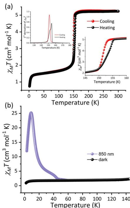
Fig. 2 (a) Temperature dependent magnetic susceptibility during cooling and heating cycles (inset: the first derivative plot and the zoomed-in view of the  $\chi_{\text{M}}T$  vs.  $T$  plot). (b) Temperature dependent susceptibility after irradiation with 850 nm light.
