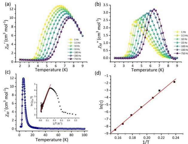
Fig. 4 AC susceptibility data collected under a 0 Oe applied dc field and a 3.5 Oe ac field oscillating at different frequencies after irradiation with 850 nm light. (a) In-phase ( $\chi'_M$ ) and (b) out-of-phase ( $\chi''_M$ ) ac susceptibility. (c)  $\chi'_M$  collected at 1 Hz. Inset represents the plot of  $\ln(\chi' T)$  versus  $T^{-1}$  (the red solid line indicates the best fit). (d) Plot of relaxation times versus  $T^{-1}$  (the red solid line indicates the best fit).
