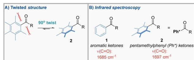
Fig. 1 General structure of pentamethylphenyl (Ph\*) ketone **2**.
