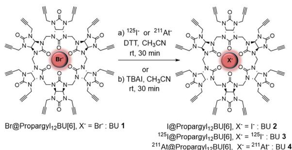
Scheme 1 Synthesis of <sup>125</sup>I@**BU 3** and <sup>211</sup>At@**BU 4** radiocomplexes (conditions a) and I@**BU 2** (conditions b).
