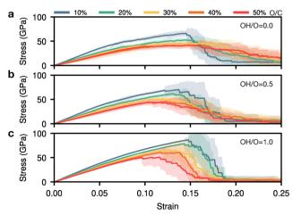
Fig. 2 Mechanical behaviour of GO and its dependence on the oxygen content. We show stress-strain curves for 20 GO sheets of  $\sim$ 200 atoms each, at varying O/C ratio (indicated by colour-coding). The shaded areas indicate one standard deviation. We characterise sheets that have been functionalised: (a) fully with epoxide groups; (b) with half epoxide, half hydroxyl groups; and (c) fully with hydroxyl groups
