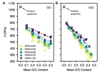
Fig. 3 Controlling the Young's modulus, E, of GO by tuning the hydroxyl content. Results are shown for varying initial OH/O ratios. (a) E values for GO: averaged for 10 structures of  $\sim$  200 atoms each, strained uniaxially in x (filled markers), and 10 strained uniaxially in y (unfilled), respectively. The cross represents pristine graphene. (b) As for panel (a), except that the structures have been thermally reduced for 10 ps.
