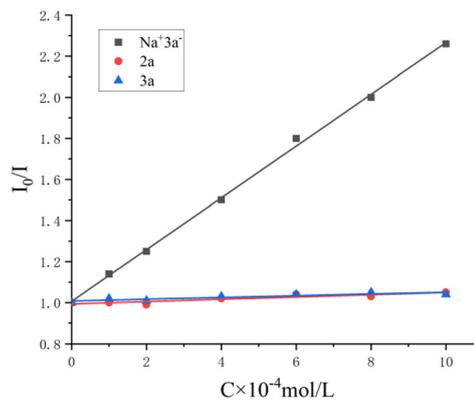
Fig. 1 Stern–Volmer plots.  $I_0$  is the inherent fluorescence intensity of [Ir(dtbbpy)(ppy)<sub>2</sub>]PF<sub>6</sub>.  $I$  is the fluorescence intensity of [Ir(dtbbpy)(ppy)<sub>2</sub>]PF<sub>6</sub> in the presence of Na<sup>+</sup>3a<sup>-</sup>, **2a** or **3a**.
