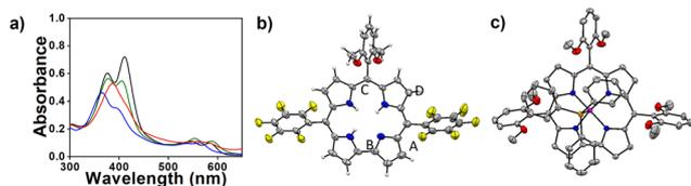
**Fig. 1** The (a) electronic spectra (in ethyl acetate) of the (triphenylphosphine)cobalt(III) corroles **1a** (black), **1b** (green), **1c** (blue), and **1d** (red) and ORTEP presentation (pink-cobalt, blue-nitrogen, gray-carbon, red-oxygen, orange-phosphorus) of the X-ray crystal structures obtained for (b) the metal-free corrole of complex **1b** and (c) complex **1c**.
