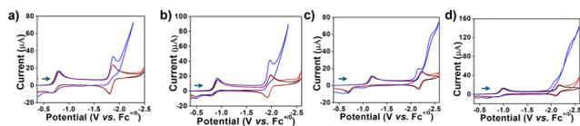
Fig. 3 Cyclic voltammograms recorded for (a) **1a**, (b) **1b**, (c) **1c** and (d) **1d** dissolved in anhydrous CH<sub>3</sub>CN under N<sub>2</sub>, 1% H<sub>2</sub>O under N<sub>2</sub>, and 1% H<sub>2</sub>O under CO<sub>2</sub> (the black, red and blue traces, respectively).
