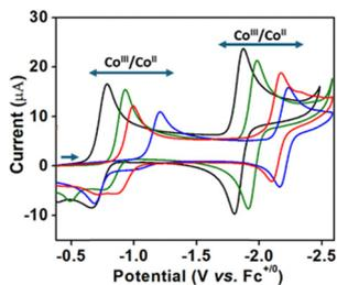
Fig. 2 Cyclic voltammograms ( $100 \text{ mV s}^{-1}$ ) of the Co corrole complexes (1 mM) **1a** (black), **1b** (green), **1c** (blue), and **1d** (red) in anhydrous MeCN/TBAPF<sub>6</sub>, 0.1 M electrolyte solution under N<sub>2</sub> atmosphere.
