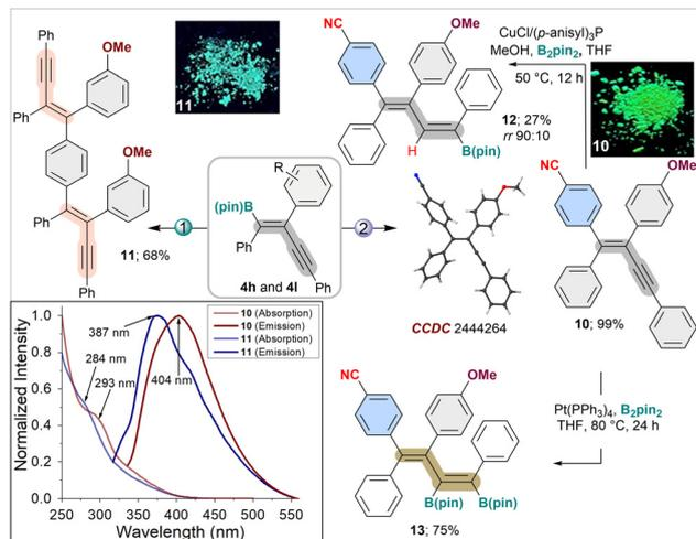
**Scheme 2** Synthetic utility of **4h** and **4l** (1) **4h** (2.2 equiv.), Pd(OAc)<sub>2</sub> (10 mol%), SPhos (20 mol%), 1,4-diiodobenzene (1 equiv.), KOH (6 equiv.), THF, 70 °C, 24 h. (2) **4l** (1 equiv.), Pd(OAc)<sub>2</sub> (5 mol%), SPhos (10 mol%), 4-iodobenzonitrile (1.2 equiv.), KOH (3 equiv.), THF, 70 °C, 24 h.
