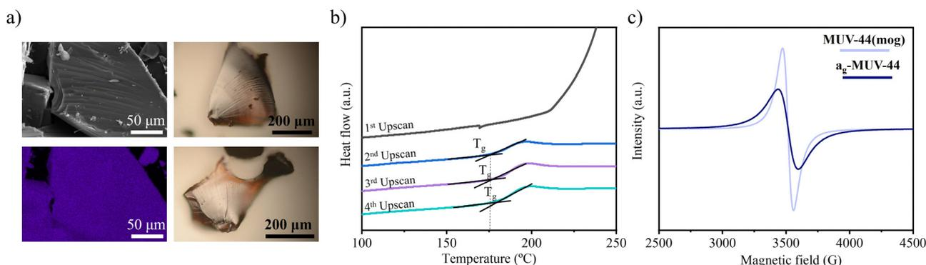
**Fig. 3** (a) SEM image of the **ag-MUV-44** monolith (left, top) accompanied by Mn elemental analysis mapping (left, bottom), along with two microscope images of different glassy samples (right). (b) Successive DSC upscans reveal the phase transition from **mog** to **dia-c** in the first upscan, while in subsequent upscans, the  $T_g$  is determined. (c) EPR spectra of **MUV-44(mog)** and **ag-MUV-44**.
