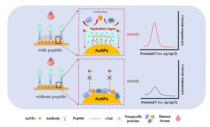
Fig. 5 Example of how peptides can introduce a hydration layer, preventing biofouling on an electrode surface. Schematic mechanism of the electrochemical immunosensor for cTnl detection based on CEAK16 peptide. Abbreviations: cTnl, cardiac troponin I; AuNPs, gold nanoparticles. Reproduced from ref. 125 with permission from publisher Elsevier, copyright 2024.
