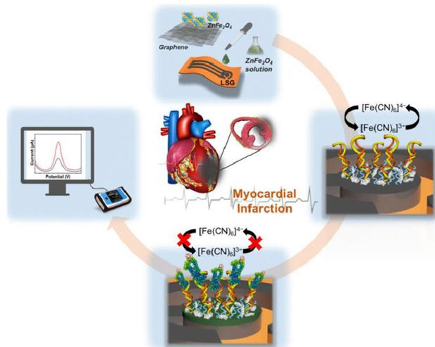
Fig. 4 Schematic overview of aptasensors. This example shows a laser-scribed graphene electrochemical aptasensor, modified with metal oxides for sensitive AMI screening. Reproduced from ref. 118 with permission from Elsevier, copyright 2021.
