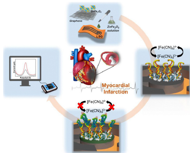
Fig. 4 Schematic overview of aptasensors. This example shows a laser-scribed graphene electrochemical aptasensor, modified with metal oxides for sensitive AMI screening. Reproduced from ref. 118 with permission from Elsevier, copyright 2021.
