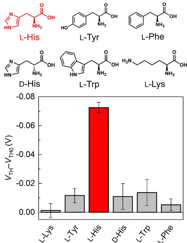
Fig. 4 Selectivity test results of the MIP-OFET for amino acids (1.0 mM) in a phosphate buffer solution (100 mM) at pH 6.0 at 25 °C. The terms  $V_{TH0}$  and  $V_{TH}$  mean threshold voltages before and after adding targets ( $n = 3$ ).
