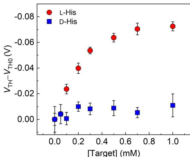
Fig. 3 Responses of the MIP-OFET to *L*-His (red circles) and *D*-His (blue squares) in a phosphate buffer solution (100 mM) at pH 6.0 at 25 °C. The terms  $V_{TH0}$  and  $V_{TH}$  mean threshold voltages before and after adding targets ( $n = 3$ ). The titration isotherms were obtained by collecting  $V_{TH}$ s at  $V_{GS} = -2$  V.
