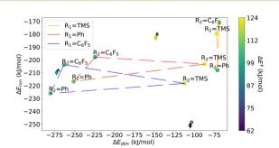
Fig. 3  $\omega$ B97X-D/6-311++G(d,p) dimerization energies ( $\Delta E_{dim}$ ) shown together with the C-H bond activation energy ( $\Delta E_{rxn}$ ) and barrier ( $\Delta E^{\ddagger}$ ).  $R_1$  and  $R_2$  groups are defined in Fig. 1, whereas structure  ${\bf A}$ ,  ${\bf B}$ , and  ${\bf D}$  are shown in Fig. 2. The proxy to the imide proposed by Nikonov et al. is  $R_1$  = Ph,  $R_2 = TMS.^{25}$
