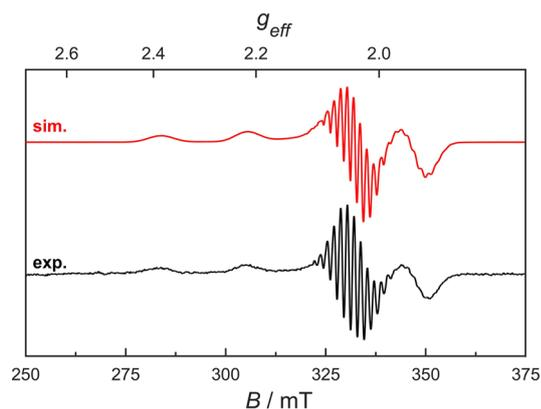
Fig. 2 EPR-spectrum of a 1.34 mM frozen solution (at  $T = 148$  K) of **Cuby** in  $\text{H}_2\text{O}$ :glycerol (4 : 1) and its simulation with key parameters obtained by least square fitting (for details see the ESI,† Table S1). The spectra exhibited a significant T-dependence, with a maximum signal intensity of around 200 K and continuous decrease at lower temperatures (see the ESI,† Fig. S4).
