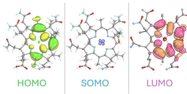
Fig. 4 Frontier molecular orbitals (FMOs) of the cupribyric acid cation (**HCuby**<sup>+</sup>) from the self-consistent field in gas-phase calculations. From left to right: the highest occupied MO (HOMO), a corrin  $\pi$ -type orbital; the  $d_{x^2-y^2}$ -type Cu(II)-located singly occupied MO (SOMO); and the lowest unoccupied MO (LUMO), a corrin  $\pi$ -type orbital. Orbitals are seen from the upper side.
