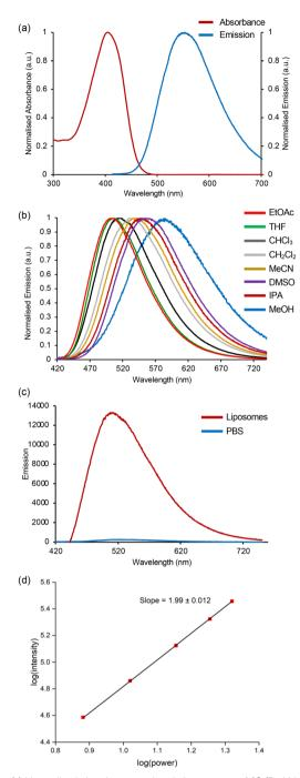
Fig. 2 (a) Normalised absorbance and emission spectra of 12 (5  $\mu$ M in DMSO). (b) Normalised emission spectra of 12 in various solvents (5  $\mu$ M). (c) Emission spectrum of 12 in liposomes (PC: cholesterol, 7:1) versus PBS (5 μM). (d) Log-log plot of fluorescence intensity *versus* laser power for **12** in DMSO ( $\lambda_{Ex}$  = 800 nm).
