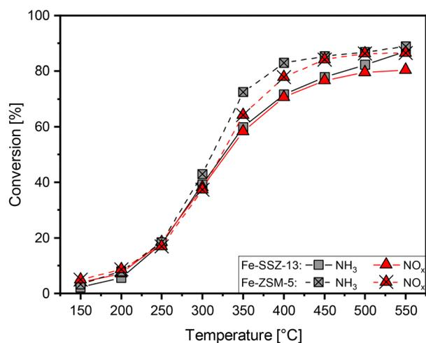
Fig. 6 Conversion of  $\text{NH}_3$  (black line) and  $\text{NO}_x$  (red line) during  $\text{NH}_3$ -SCR over Fe-ZSM-5 (dashed lines) and Fe-SSZ-13 (solid lines) synthesized by improved ion exchange after hydrothermal aging (10%  $\text{H}_2\text{O}$ , 10%  $\text{O}_2$  in  $\text{N}_2$ ) at 650 °C for 16 h. Gas composition: 350 ppm NO, 350 ppm  $\text{NH}_3$ , 12%  $\text{H}_2\text{O}$ , 10%  $\text{O}_2$  in  $\text{N}_2$ .
