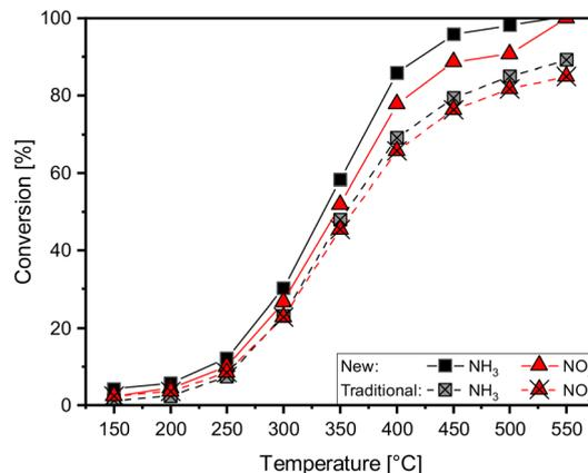
Fig. 5 Conversion of  $\text{NH}_3$  (black line) and  $\text{NO}_x$  (red line) during  $\text{NH}_3$ -SCR over Fe-SSZ-13 synthesized by improved and traditional ion exchange. Gas composition: 350 ppm NO, 350 ppm  $\text{NH}_3$ , 12%  $\text{H}_2\text{O}$ , 10%  $\text{O}_2$  in  $\text{N}_2$ .
