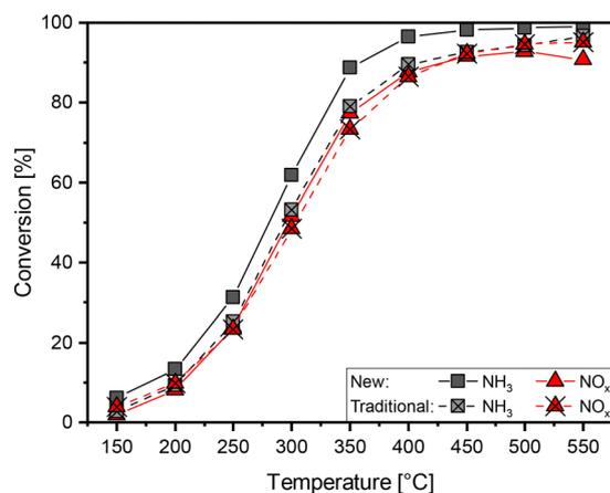
Fig. 4 Conversion of  $\text{NH}_3$  (black line) and  $\text{NO}_x$  (red line) during  $\text{NH}_3$ -SCR over Fe-ZSM-5 synthesized by improved and traditional ion exchange. Gas composition: 350 ppm NO, 350 ppm  $\text{NH}_3$ , 12%  $\text{H}_2\text{O}$ , 10%  $\text{O}_2$  in  $\text{N}_2$ .
