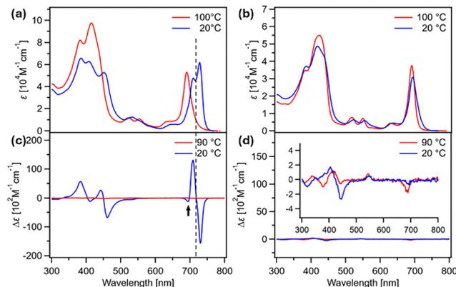
**Fig. 2** (a) and (b) Changes in the UV/Vis absorption and (c) and (d) CD spectra of (a) and (c) **Chl<sub>d</sub>** (100  $\mu\text{M}$ ) and (b) and (d) **Chl<sub>m</sub>** (300  $\mu\text{M}$ ) upon cooling from 100 to 20 °C at a rate of  $1 \text{ }^\circ\text{C min}^{-1}$  in MCH.
