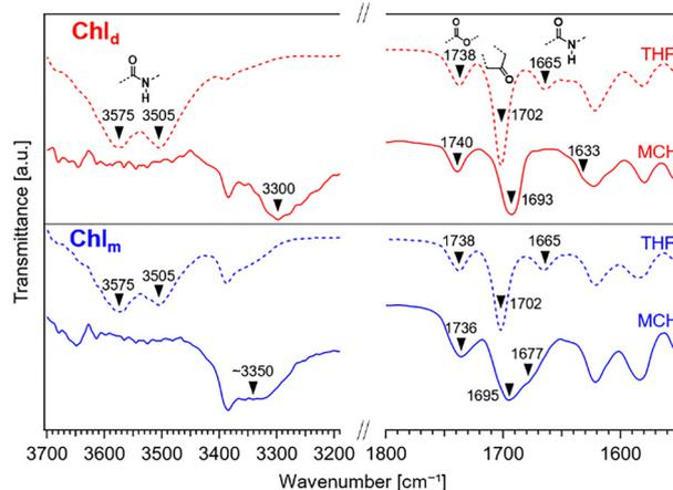
**Fig. 4** FT-IR spectra of **Chl<sub>d</sub>** (*c* = 200 μM, upper) and **Chl<sub>m</sub>** (*c* = 1.2 mM, lower) in THF (dashed lines) and MCH (solid lines).
