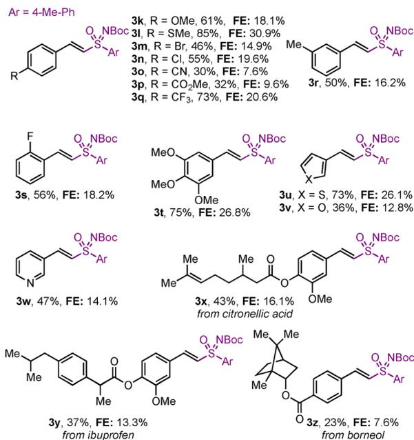
**Scheme 2** Substrates scope; **1** (0.2 mmol), **2** (3.0 equiv.) and K<sub>2</sub>CO<sub>3</sub> (4.0 equiv.) in MeCN : H<sub>2</sub>O (10 : 1, 2.0 mL) were electrolyzed at 3 mA CCE using GF (anode) and Ni (cathode) under argon. FE = faradaic efficiency.
