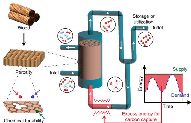
Fig. 8 Schematic showing the steam-assisted temperature vacuum swing desorption process with wood-derived AC as the CO<sub>2</sub> adsorbent. Graphene-derived materials are suitable templates for evaluating AC-based materials. Integrating with a dynamic energy supply results in energy- and cost-effective solutions for carbon capture. Figure is reproduced with permission from ref. 94 under a Creative Commons License CC BY 4.0.
