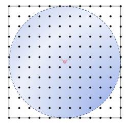
Fig. 2 An example for the real-space grids representation, where  $R_{\rm cut}$  is shown by the blue sphere. The wave function is set to zero outside the sphere. Figure is reproduced with permission from ref. 24 under a Creative Commons License CC BY 4.0.
