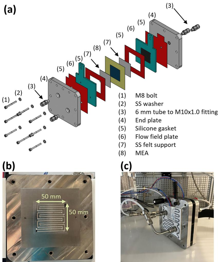
Fig. 5 (a) Detailed view of the EHP showing all components of the test cell; (b) and (c) photographs of the 25 cm<sup>2</sup> double serpentine flow field plate design and the fully assembled EHP, respectively.
