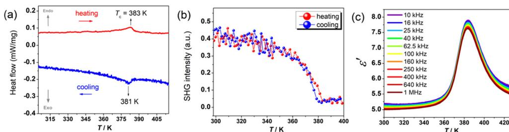
**Fig. 3** Thermal, optical, and dielectric properties of 2-ADAB. (a) DSC curves showing a reversible phase transition near 383 K. (b) Temperature-dependent SHG intensity, confirming the noncentrosymmetric nature of ferroelectric phase. (c) The temperature-dependent dielectric constant ( $\epsilon'$ ) measured on a pressed-powder pellet during the heating run.
