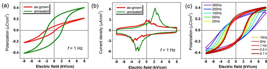
Fig. 4 Polarization switching behaviour of 2-ADAB single crystals. (a)  $P$ - $E$  hysteresis loops for the as-grown state and the annealed states at 298 K (b) Current density-electric field curves. (c) Frequency-dependent  $P$ - $E$  hysteresis loops for annealed sample measured under an applied electric field.
