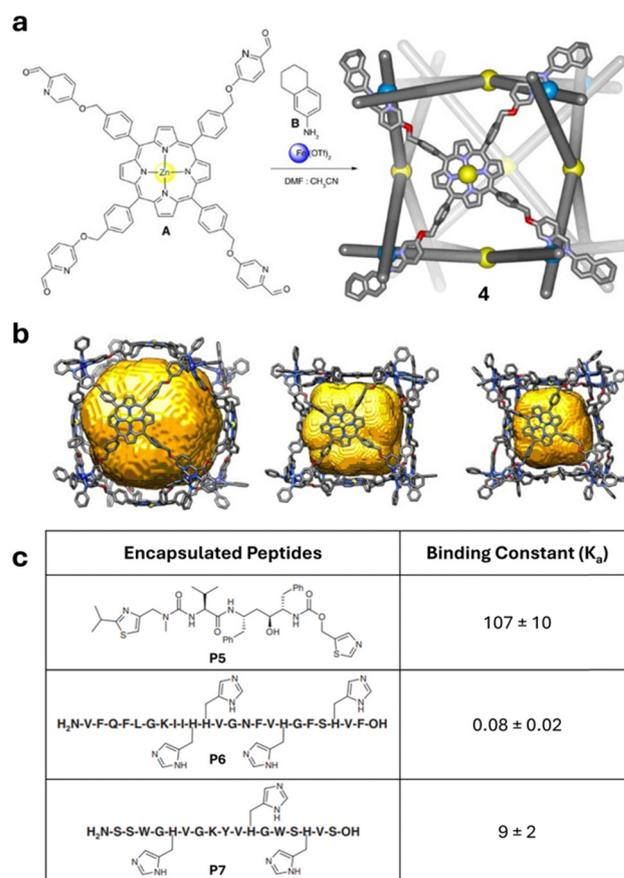
Fig. 4 (a) Self-assembly of **4**, a cubic MOC with one zinc porphyrin per face; (b) MM2 energy minimised models of **4** showing the structural flexibility and variable void volumes from 10 083 to 3143 Å<sup>3</sup>; (c) peptides **P5–P7** found to bind within **4** and their binding constants. Reproduced with permission from ref. 6.
