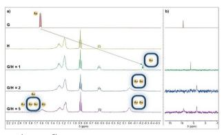
Fig. 4 <sup>1</sup>H (a) and <sup>31</sup>P NMR (b) spectra of **G**, **H** and **G/H** mixtures of different ratios
