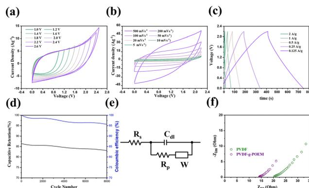
**Fig. 3** (a) Cyclic voltammetry of the prepared EDLC cells with different voltage windows and (b) with different scan rates, (c) GCD curves of the EDLC cells, (d) stability test of the prepared cell based on amphiphilic PVDF-*g*-POEM double comb copolymers, (e) graph of the representative equivalent circuit, and (f) Nyquist plot of the EDLC cell based on hydrophobic PVDF and amphiphilic PVDF-*g*-POEM double comb copolymers.
