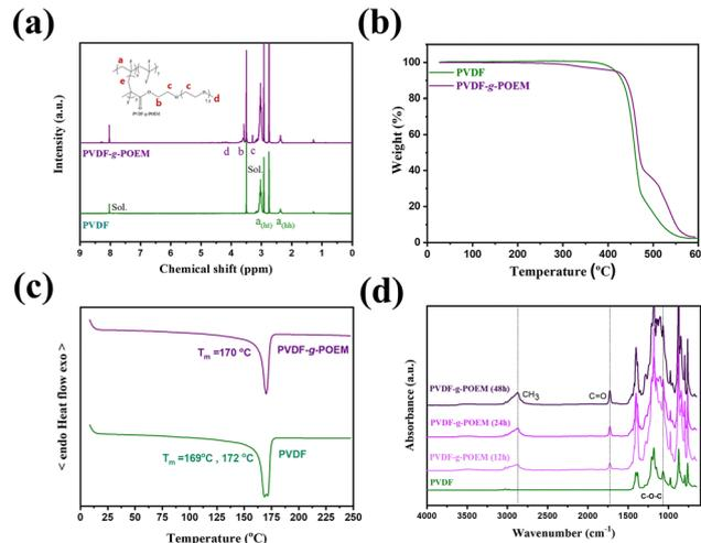
Fig. 1 (a) <sup>1</sup>H-NMR spectra of the hydrophobic PVDF and amphiphilic PVDF-*g*-POEM double comb copolymer and (b) TGA curves of the polymer under air conditions. (c) 2nd cycle of the DSC curves of the hydrophobic PVDF and amphiphilic PVDF-*g*-POEM double comb copolymer. And (d) FT-IR spectra of the hydrophobic PVDF and amphiphilic PVDF-*g*-POEM double comb copolymer with different reaction periods.
