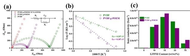
**Fig. 2** (a) Nyquist plot of EIS obtained from stainless blocking electrodes for ionic conductivity measurement with an inset showing the simplified RC circuit for solid-state electrolytes. (b) Arrhenius plot of the solid-state electrolytes prepared with 15 wt% LiTFSI content. (c) Bar graphs showing measured ionic conductivity of the solid-state electrolytes prepared from hydrophobic PVDF and amphiphilic PVDF-*g*-POEM double comb copolymer with various LiTFSI contents.
