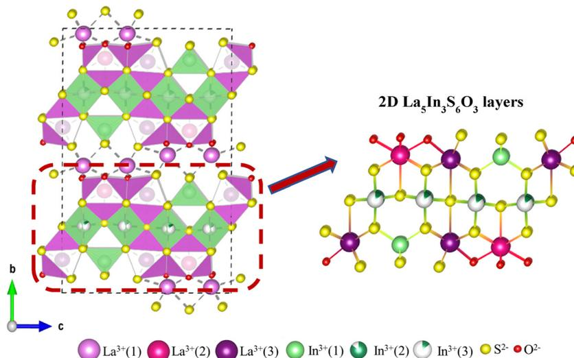
Fig. 6 Structural representation of  $\text{La}_5\text{In}_3\text{S}_9\text{O}_3$  oxysulfide ( $Pbcm$  symmetry) with the 2D  $\text{La}_5\text{In}_3\text{S}_6\text{O}_3$  layers consisting of two building blocks: rock-salt layers formed by both indium and lanthanum and fluorite-type ribbons formed by lanthanum atoms; alternating regularly along  $b$ .
