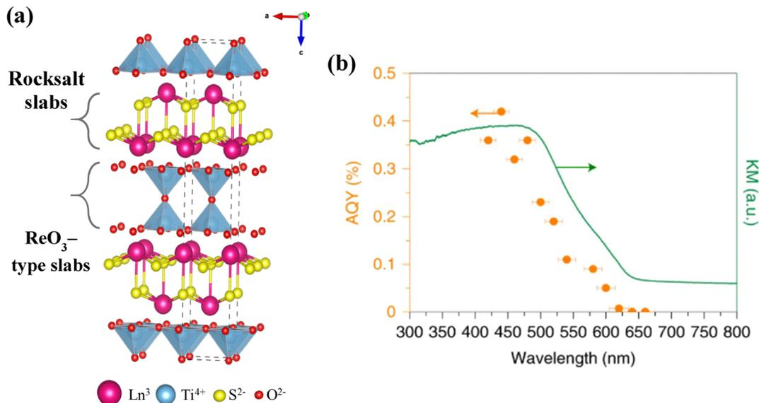
Fig. 3 (a) Structural representation of the Ruddlesden–Popper structure of the  $Ln_2Ti_2S_2O_5$  series of  $I4/mmm$  symmetry; (b) shows apparent quantum yield (AQY) for overall water splitting and diffuse reflectance spectrum (DRS) measured for  $Cr_2O_3/Rh/IrO_2$ -modified  $Y_2Ti_2O_5S_2$ . Reproduced from ref. 85 with permission from Springer Nature.
