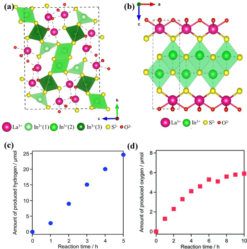
Fig. 5 Structural representation of LaOInS<sub>2</sub> material with (a) alpha model of *Pbcm* symmetry and (b) metastable layered model of *P21/m* symmetry; below, the water splitting properties of the metastable layered phase of LaOInS<sub>2</sub> are shown including (c) H<sub>2</sub>(g) evolution for 0.75 wt% Pt/LaOInS<sub>2</sub> and (d) O<sub>2</sub>(g) evolution for 0.5 wt% IrO<sub>2</sub>/LaOInS<sub>2</sub>. Reproduced from ref. 95 with permission from the Royal Society of Chemistry.
