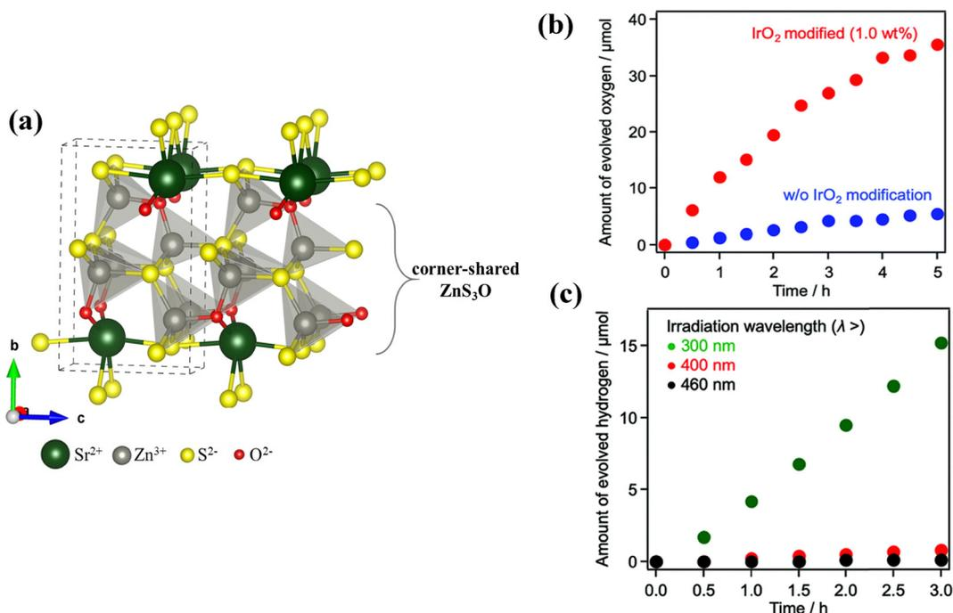
**Fig. 4** (a) Structural representation of  $\text{SrZn}_2\text{S}_2\text{O}$  oxysulfide of  $Pmn2_1$  symmetry; (b) oxygen evolution for  $\text{SrZn}_2\text{S}_2\text{O}$  and (c) hydrogen evolution for Pt/ $\text{SrZn}_2\text{S}_2\text{O}$ . Reproduced from ref. 92 with permission from the Royal Society of Chemistry.
