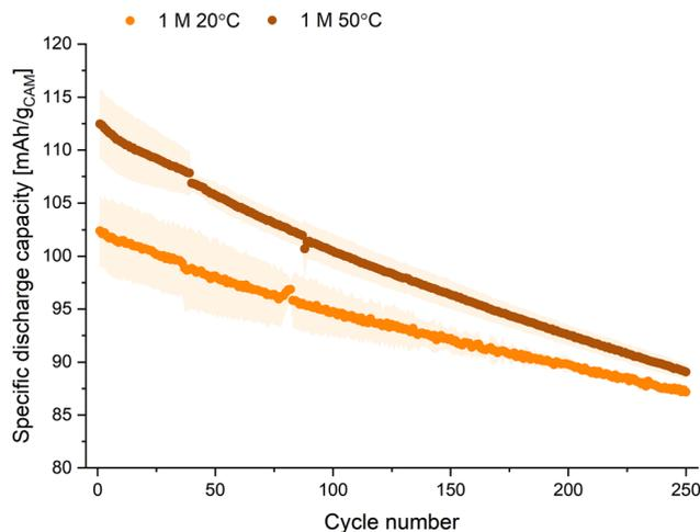
Fig. 4 Comparison of specific discharge capacity vs. cycle number at 20 °C and 50 °C for 1 M NaPF<sub>6</sub> in EC:DEC (1:1 v/v) electrolyte. The applied C-rate (C/2) was based on the expected capacity of 138 mA h g<sup>-1</sup> of the NFM111 cathode, using cell voltage limits of 1.5 and 4.0 V. Error bars display standard deviation of 2-coin cells.
