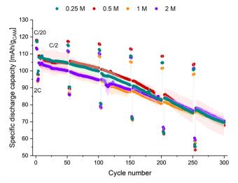
Fig. 3 Specific discharge capacity vs. cycle number using NFM111 cathode and hard-carbon anode. The applied C-rates of C/20, 2C, and C/2 were calculated based on the expected capacity of 138 mA h g $^{-1}$  of the cathode, using cell voltage limits of 1.5 and 4.0 V. Electrolyte is 0.25 M (green), 0.5 M (red), 1 M (orange) and 2 M (purple) NaPF $_6$  in EC:DEC (1:1 v/v). Error bars display standard deviation of 2–4 coin cells, cycled at 21 °C.
