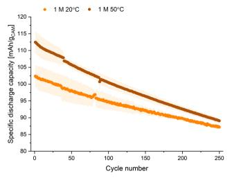
Fig. 4 Comparison of specific discharge capacity vs. cycle number at 20 °C and 50 °C for 1 M NaPF<sub>6</sub> in EC: DEC (1:1 v/v) electrolyte. The applied C-rate (C/2) was based on the expected capacity of 138 mA h g  $^{-1}$  of the NFM111 cathode, using cell voltage limits of 1.5 and 4.0 V. Error bars display standard deviation of 2-coin cells.
