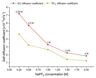
Fig. 2 Self-diffusion coefficients of the EC solvent molecule (red, <sup>1</sup>H DOSY NMR) and the  $PF_6^-$  anion (yellow,  $^{19}F$  DOSY NMR) of 0.25–2 M NaPF<sub>6</sub> in EC: DEC (1:1 v/v) electrolytes.
