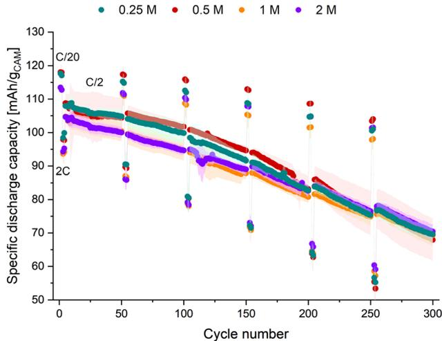
Fig. 3 Specific discharge capacity vs. cycle number using NFM111 cathode and hard-carbon anode. The applied C-rates of C/20, 2C, and C/2 were calculated based on the expected capacity of 138  $\text{mA h g}^{-1}$  of the cathode, using cell voltage limits of 1.5 and 4.0 V. Electrolyte is 0.25 M (green), 0.5 M (red), 1 M (orange) and 2 M (purple)  $\text{NaPF}_6$  in EC:DEC (1 : 1 v/v). Error bars display standard deviation of 2–4 coin cells, cycled at 21 °C.
