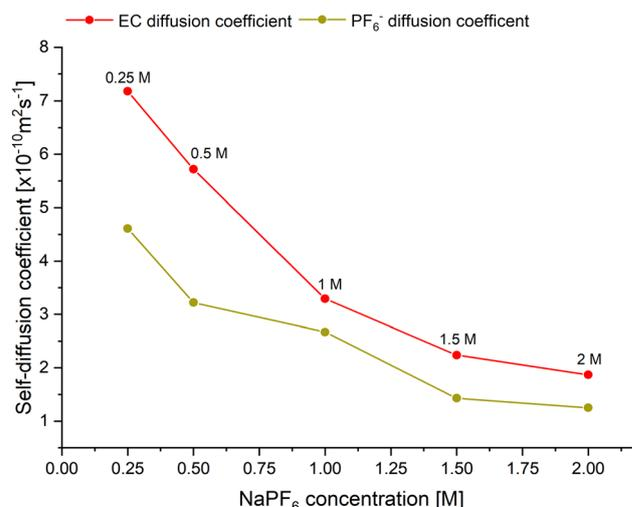
Fig. 2 Self-diffusion coefficients of the EC solvent molecule (red, <sup>1</sup>H DOSY NMR) and the PF<sub>6</sub><sup>-</sup> anion (yellow, <sup>19</sup>F DOSY NMR) of 0.25–2 M NaPF<sub>6</sub> in EC:DEC (1:1 v/v) electrolytes.
