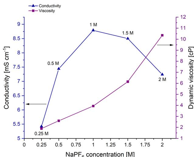
Fig. 1 Bulk conductivity (blue) and dynamic viscosity values (purple) of 0.25 M, 0.5 M, 1 M, 1.5 M and 2 M NaPF<sub>6</sub> in EC:DEC (1:1 v/v) electrolytes at approximately 25 °C.
