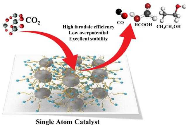
Fig. 6 Schematic illustration of SAC-derived CO<sub>2</sub> electroreduction into value-added chemicals.
