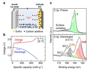
Fig. 4 (a) Schematic of a prototype Ca metal battery using an electrolyte of 0.4 M Ca(CB<sub>11</sub>H<sub>12</sub>)<sub>2</sub> with 0.05 M CaBr<sub>2</sub> in G2. (b) Voltage profile during the first cycle. (c) S 2p spectra of S/C electrodes in pristine (top) and discharged (bottom) states.
