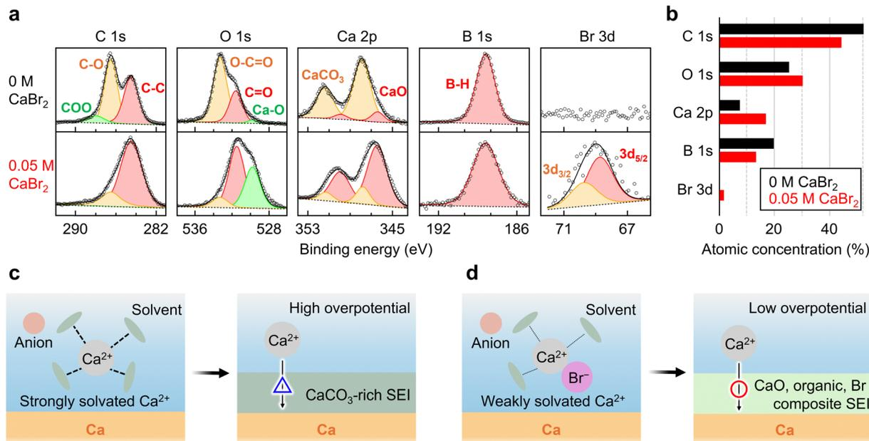
Fig. 3 (a) C 1s, O 1s, Ca 2p, B 1s, and Br 3d spectra of Ca metal soaked for 30 min in 0.4 M Ca(CB<sub>11</sub>H<sub>12</sub>)<sub>2</sub> with 0 and 0.05 M CaBr<sub>2</sub> in G2. (b) Atomic concentration (atom%) of the passivation layer components on the Ca metal surface. (c) and (d) Schematics of solvation structure and SEI formation in electrolytes (c) without and (d) with CaBr<sub>2</sub>.
