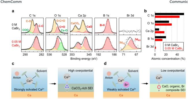
Fig. 3 (a) C 1s, O 1s, Ca 2p, B 1s, and Br 3d spectra of Ca metal soaked for 30 min in 0.4 M Ca(CB<sub>11</sub>H<sub>12</sub>)<sub>2</sub> with 0 and 0.05 M CaBr<sub>2</sub> in G2. (b) Atomic concentration (atom%) of the passivation layer components on the Ca metal surface. (c) and (d) Schematics of solvation structure and SEI formation in electrolytes (c) without and (d) with CaBr<sub>2</sub>.
