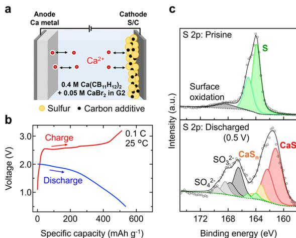
**Fig. 4** (a) Schematic of a prototype Ca metal battery using an electrolyte of 0.4 M  $\text{Ca}(\text{CB}_{11}\text{H}_{12})_2$  with 0.05 M  $\text{CaBr}_2$  in G2. (b) Voltage profile during the first cycle. (c) S 2p spectra of S/C electrodes in pristine (top) and discharged (bottom) states.
