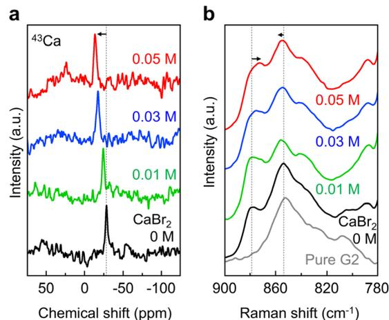
**Fig. 2** Coordination environment investigation of  $\text{Ca}^{2+}$  in 0.4 M  $\text{Ca}(\text{CB}_{11}\text{H}_{12})_2$  with 0, 0.01, 0.03, and 0.05 M  $\text{CaBr}_2$  in G2. (a)  $^{43}\text{Ca}$  NMR and (b) Raman spectra.
