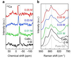
Fig. 2 Coordination environment investigation of Ca<sup>2+</sup> in 0.4 M  $Ca(CB_{11}H_{12})_2$  with 0, 0.01, 0.03, and 0.05 M  $CaBr_2$  in G2. (a)  $^{43}Ca$  NMR and (b) Raman spectra.
