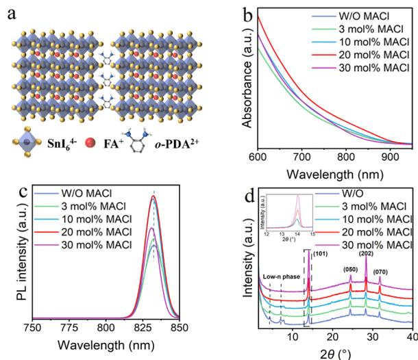
**Fig. 1** (a) Schematic representation of estimated DJ structure of quasi-2D perovskites using *o*-PDA. (b) UV-vis absorption spectra, (c) PL spectra, and (d) XRD patterns of the quasi-2D TP with different concentrations of MACl.
