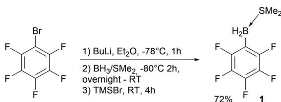
Scheme 2 Synthetic procedure for C<sub>6</sub>F<sub>5</sub>BH<sub>2</sub>·SMe<sub>2</sub> (**1**).
