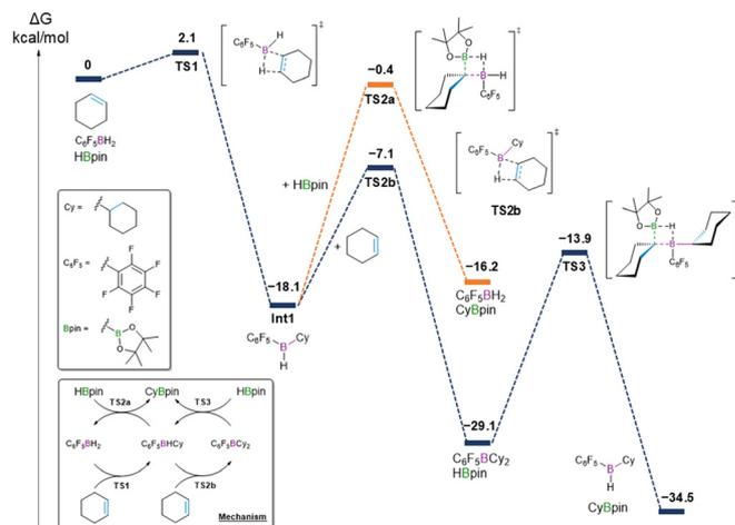
Fig. 1 Gibbs free energy diagram of the calculated reaction mechanism based on cyclohexene. The energies are given in kcal mol<sup>-1</sup> in the gas phase at 298 K. The effect of  $SMe_2$  was omitted.
