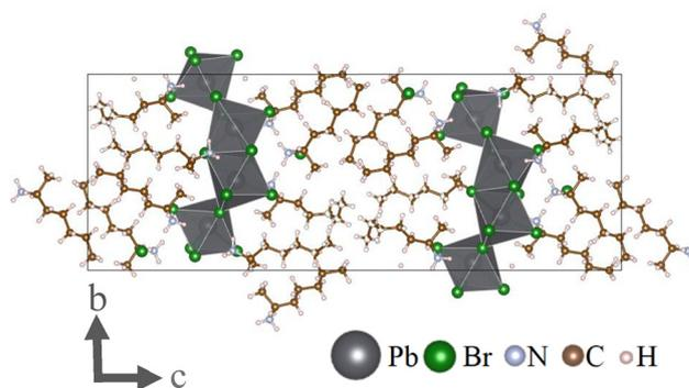
**Fig. 1** The unit cell of (S-2AH)<sub>4</sub>[Pb<sub>2</sub>Br<sub>7</sub>]Br consist of two inorganic layers made up of lead-bromide octahedra. These layers are separated by organic spacers in which a bromide anion is located. Disordered atoms omitted for clarity. This graphic was created using the VESTA software package.<sup>14</sup>
